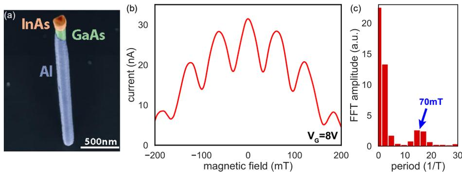
*Figure 1 (a) False-colored SEM micrograph of a GaAs/InAs/Al core/shell/halfshell nanowire. (b) Flux-dependent supercurrent oscillations induced by an in-plane magnetic field oriented along the nanowire axis. (c) FFT spectrum of the oscillations), revealing a pronounced and well-defined  $h/2e$  period for an effective radius located within the InAs shell.*
