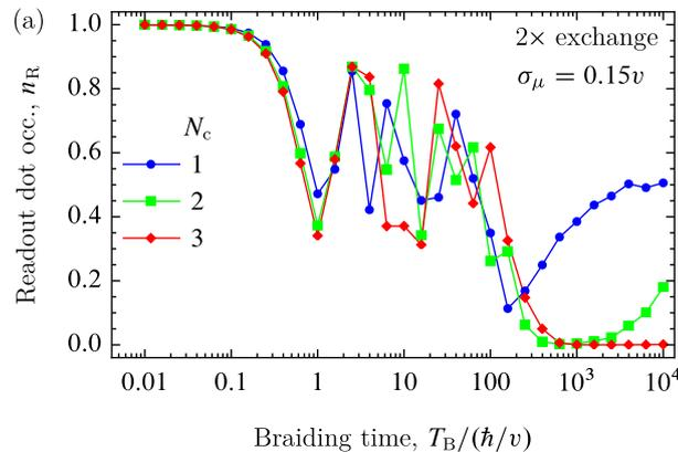
**Figure 1. Numerical demonstration of topological protection of the braiding-based quantum-logical gate.** Readout dot charge occupation as a function of the braiding time, for various system sizes ( $N_c$ ). With increased system size ( $N_c = 3$ ), a plateau emerges for long braiding times, signalling topological protection of the braiding-based quantum logical gate.
