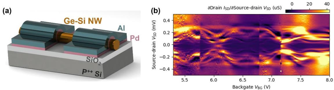
Figure 1 (a) Schematic overview of a gate tunable Ge-Si core-shell nanowire Josephson device. (b) Bias spectroscopy of the subgap states in the device.
