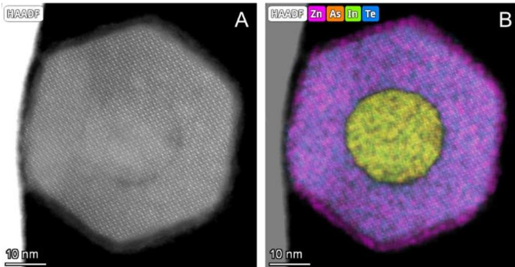
*Figure: Cross-section of a II-VI/III-V core-shell nanowire. A. High Angle Annular Dark Field TEM image. B. Chemical mapping obtained by HAADF/energy dispersive X-ray spectroscopy.*
