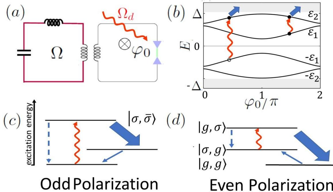
Fig: (a) Schematic setup: phase biased weak link coupled to a microwave resonator (b) Subgap states as a function of phase for a finite length weak link (c-d) Excitation of even/odd many-body states leading to polarization in the odd/even parity sector.
