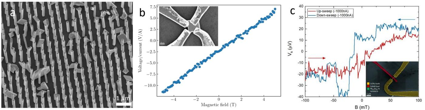
Fig. 1 (a) A representative SEM image of  $\text{Pb}_{1-x}\text{Sn}_x\text{Te}$  nanowires grown from a patterned mask. (b) A magnetoconductance graph of a  $\text{Pb}_{1-x}\text{Sn}_x\text{Te}$  nanoflake measured in the Van de Pauw configuration. The inset shows a SEM image of the measured flake. (c) The tunnel voltage measured between the ferromagnet and a metal contact as a function of the magnetic field. The inset shows a false-color SEM image of the measured device
