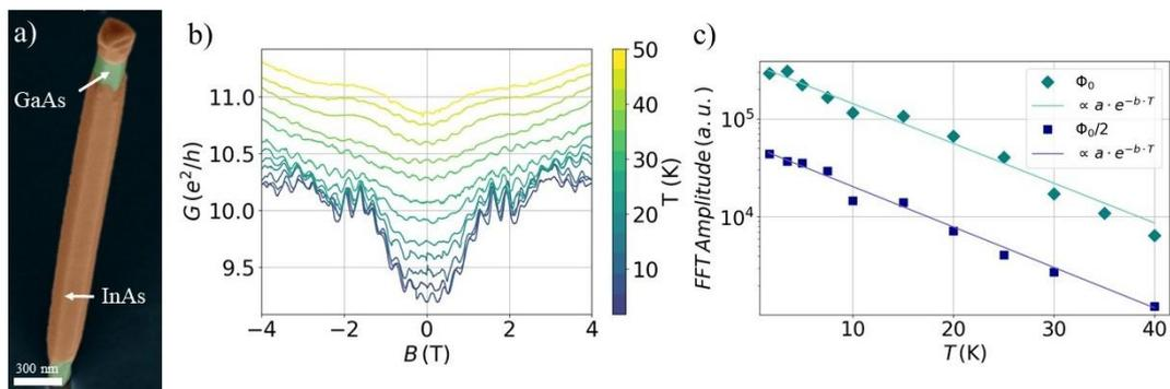
Figure 1 a) Electron micrograph of a GaAs/InAs core/shell nanowire. b) Magnetoconductance oscillations at various temperatures. c) Amplitude of Aharonov-Bohm oscillations vs. temperature and fit according to a quasi-ballistic transport regime.
